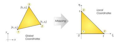
Figure 2 – Triangular element in xy and in  $\xi \eta$  spaces
