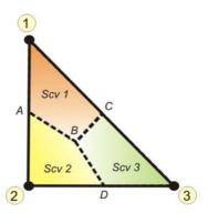
Figure 5 – Triangular element composed of three sub-control volumes (Scv)
