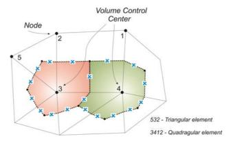
Figure 1. Example of a grid used in the CVFEM
