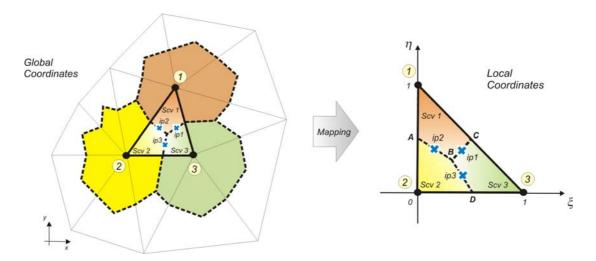
Figure 3 – Triangular element, showing its sub-control volumes (Scv) and the integration points (ip)
