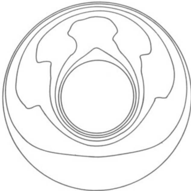
Fig. 6 - Isotherms for the concentric case
