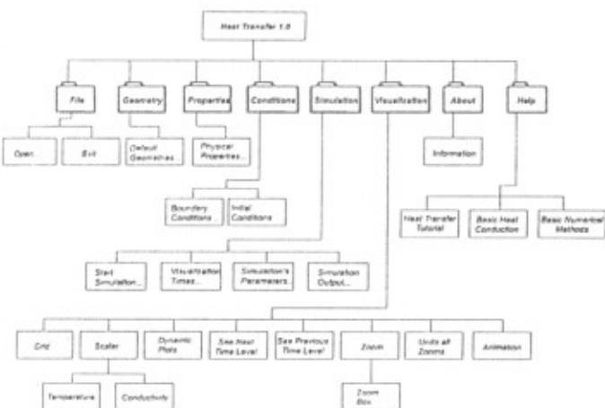
Fig. 4 - Structure of Heat Transfer 1.0
