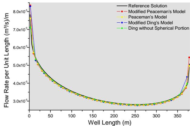
Figure 2. Horizontal Well Flow Rate Gradient - Spherical Portion Test
