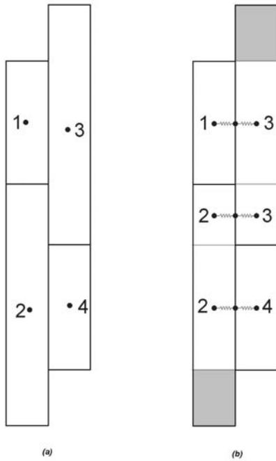
Fig. 13 – (a) Corner point grid; (b) Resistance representative scheme used in simulators where the gray areas are not utilized in the calculus of transmissibilities
