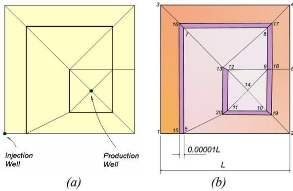
Figure 5 – ‘Labyrinth problem’ in the second case: (a) grid used, and (b) detail of the fault with its width enlarged to better the visualization
