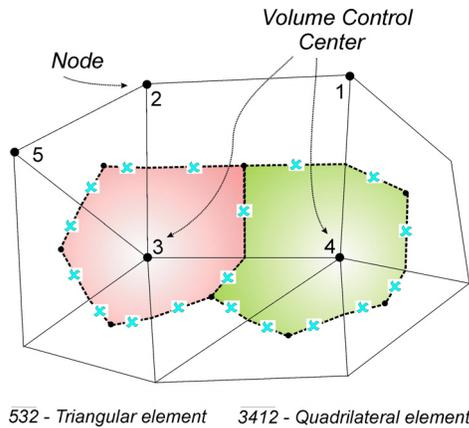
Figure 1 – Example of a grid used in the EbFVM
