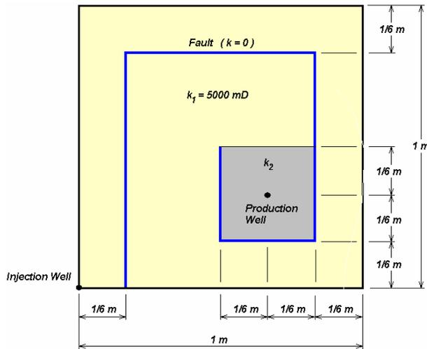
Figure 3 – Depiction of the reservoir of the Test-problem, where  $k_2$  assumes values of 5000 mD (homogeneous problem) or 50 mD (heterogeneous problem)
