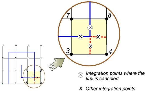
Figure 7 – Grid element showing the physical inconsistency in using the value of node 7 in the flux discretized equation at the integration points (X)
